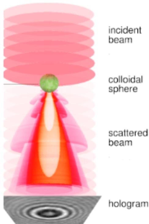
**Figure 3.** Breakdown of a H.M. demonstrating the interaction of the laser with the **colloidal sphere** and the resulting interference (hologram).
