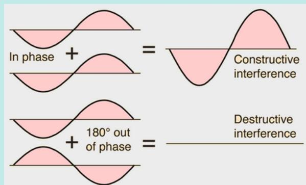
**Figure 1.** Image of destructive and constructive wave interference.
