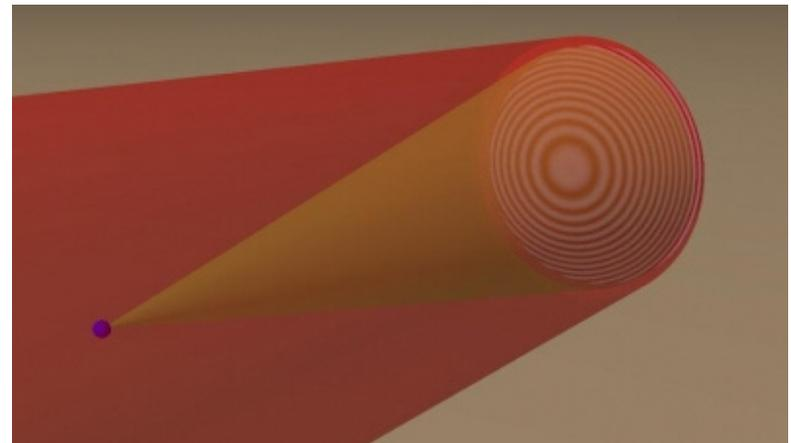
**Figure 5.** Red light is the original laser(reference beam) while the yellow light represents the object beam.
