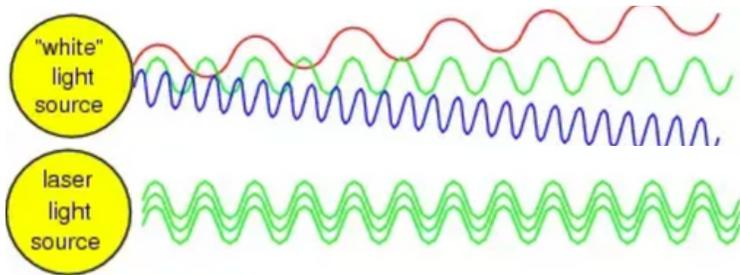
**Figure 2.** White light contains different wavelengths that travel **out of phase** with each other - waves of a laser travel **in phase** in a uniform direction.
